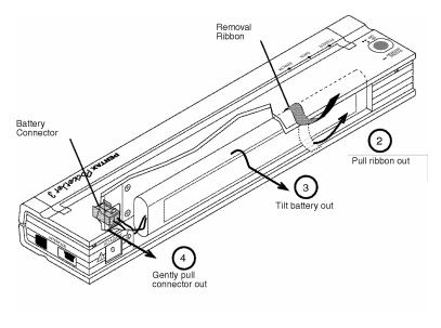
FIGURE 13. Instructions for removing the battery
